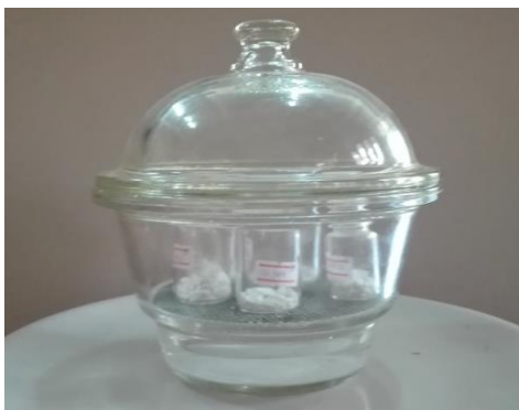
Figure 1: Photograph of the experiment for water vapour transmission of films
