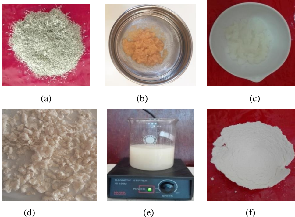
Figure 2: Photographs of (a) sawdust (b) alkali treated fiber (c) bleached pulp (d) dried pulp (e) acid hydrolysis of bleached pulp and (f) dried MFC
